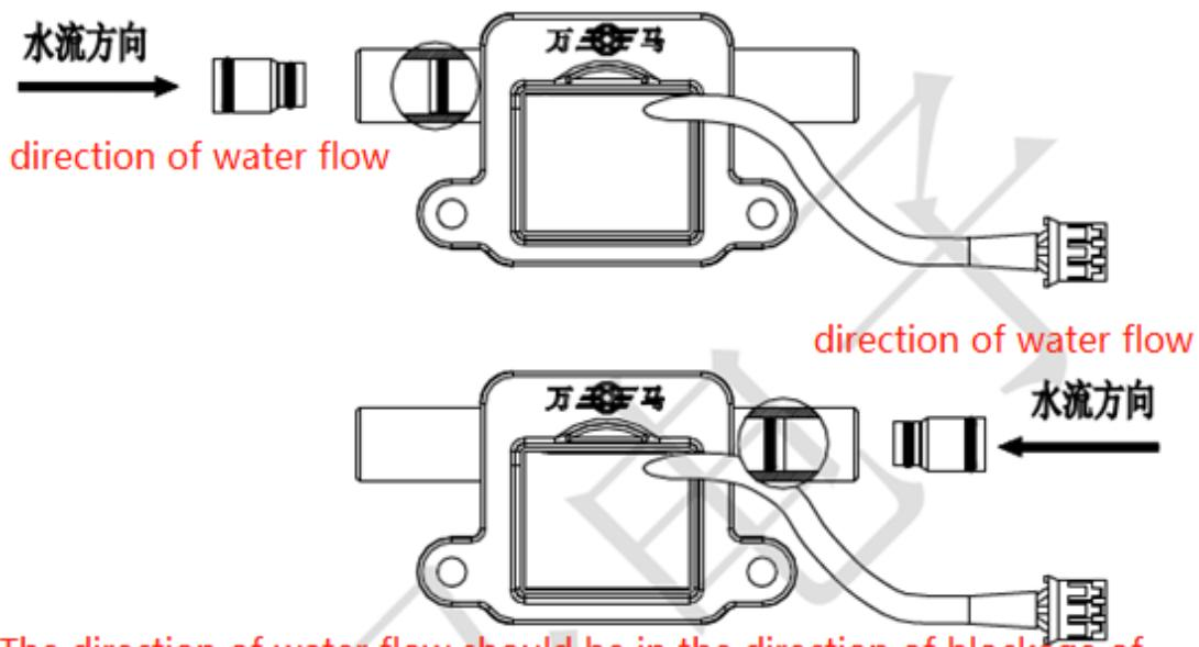
The direction of water flow should be in the direction of blockage of water inflow.
