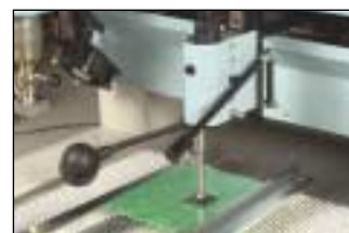
BGA placement is easy using the patented Weller® placement templates.
