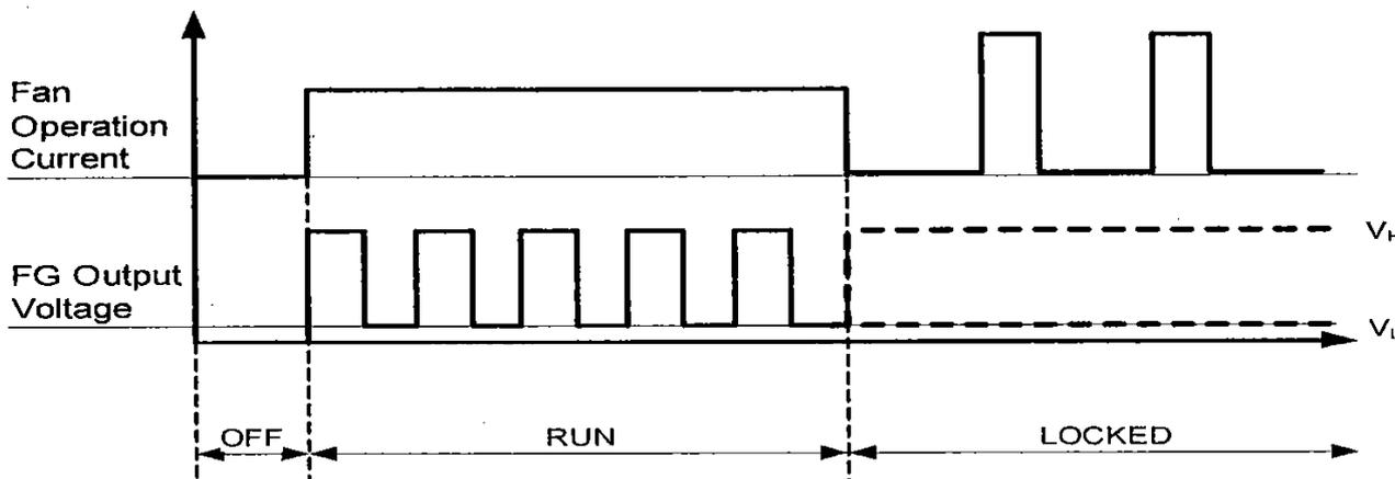
★Electrical Characteristics : ( at Ta = 25°C, V<sub>CC</sub>=3V)
