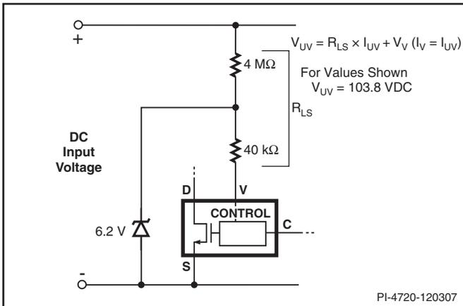
Figure 20. Line Sensing for Undervoltage Only (Overvoltage Disabled).
