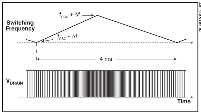
Figure 10. Switching Frequency Jitter (Idealized  $V_{DRAIN}$  Waveforms).
