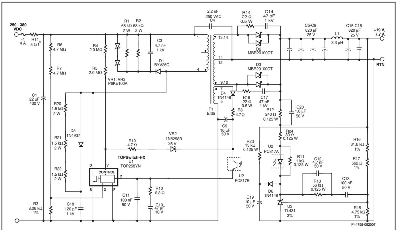
Figure 42. 150 W, 19 V Power Supply using TOP258YN.
