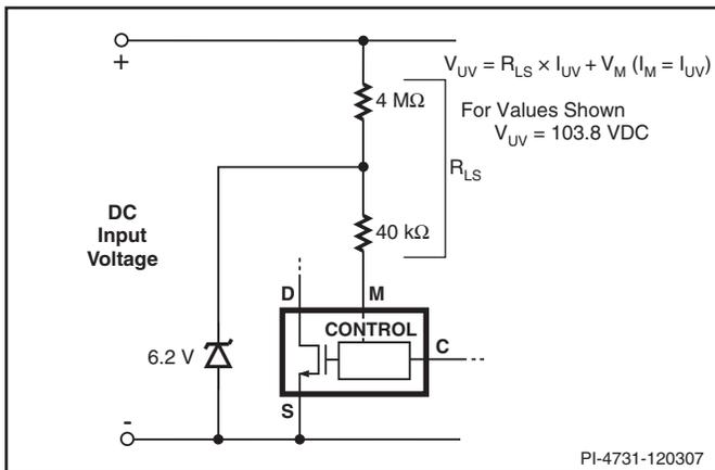
Figure 33. Line Sensing for Undervoltage Only (Overvoltage Disabled).
