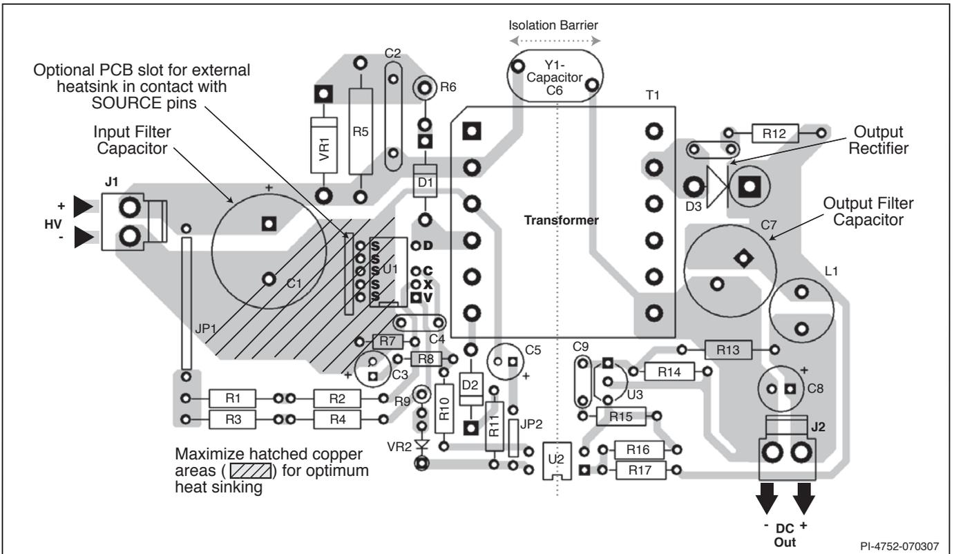
Figure 47. Layout Considerations for TOPSwitch-HX Using M-Package.
