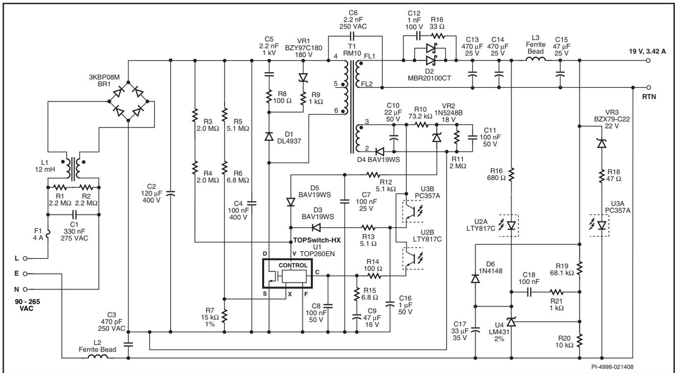
Figure 44. 65 W, 19 V Power Supply Using TOP260EN.
