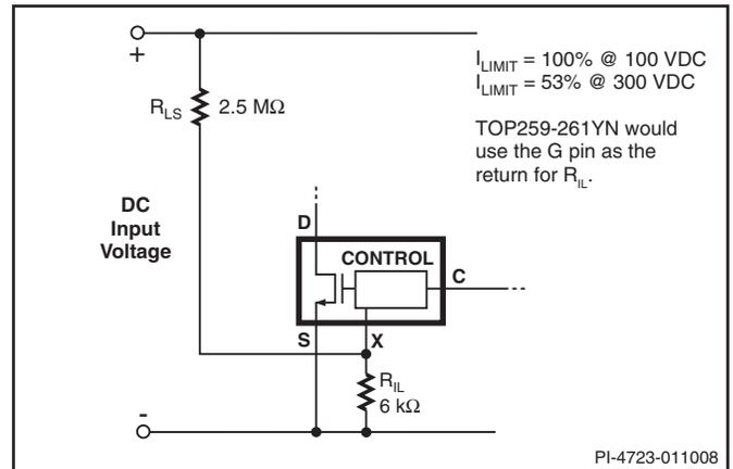
Figure 23. Current Limit Reduction with Line Voltage.
