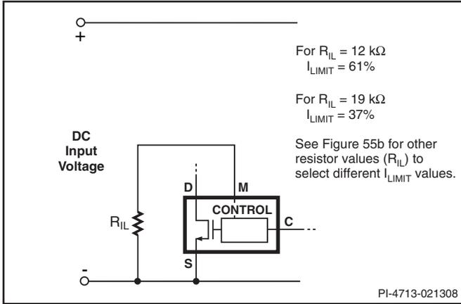
Figure 8. P/G Package Externally Set Current Limit.
