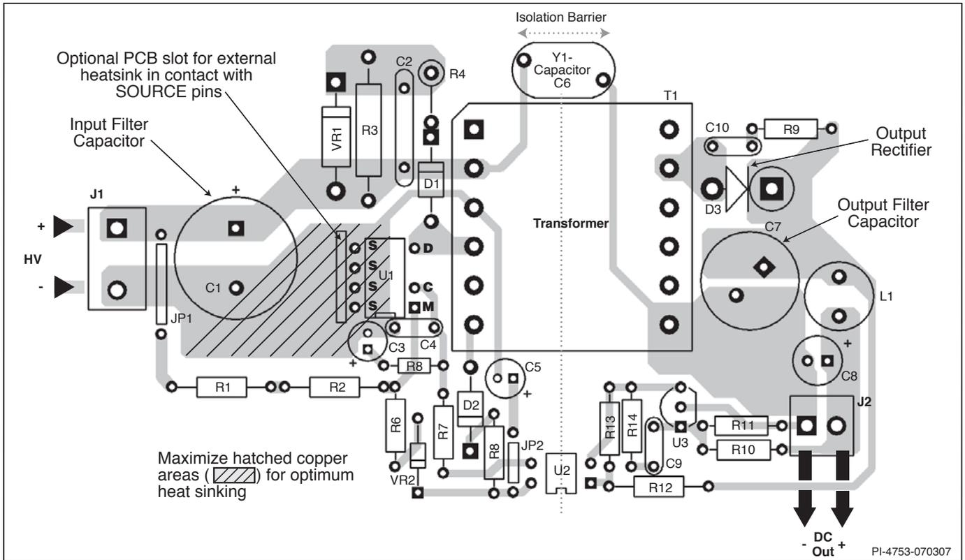
Figure 46. Layout Considerations for TOPSwitch-HX Using P-Package.
