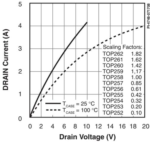
Figure 66. Output Characteristics.
