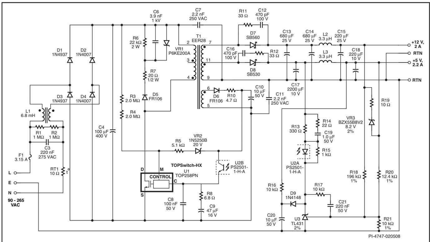
Figure 41. 35 W Dual Output Power Supply using TOP258PN.
