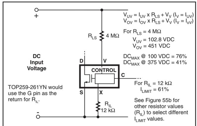
Figure 27. Line Sensing and Externally Set Current Limit.
