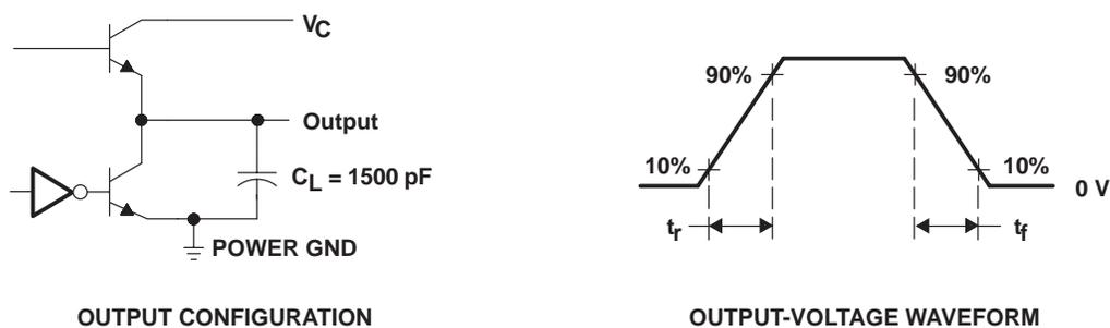
Figure 2. Switching Output Configuration and Voltage Waveform
