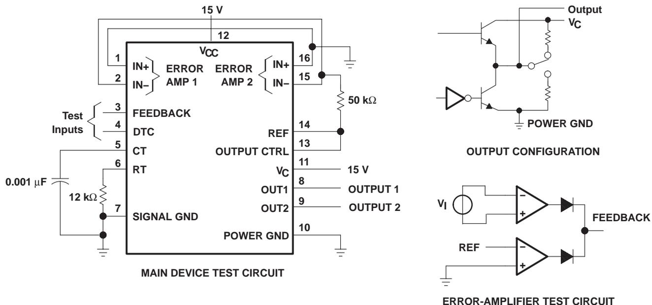
Figure 1. Test Circuits
