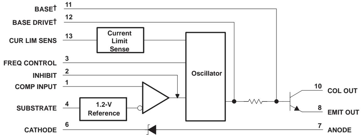
† BASE and BASE DRIVE are used for device testing only. They normally are not used in circuit applications of the device.
