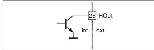
Non-conductive state of HOT (Horizontal Output Transistor) must correspond to non-conductive state of the device output transistor.
