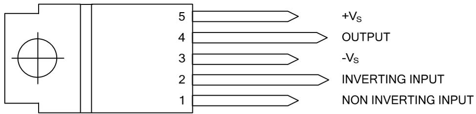
\*TAB CONNECTED TO PIN 3
