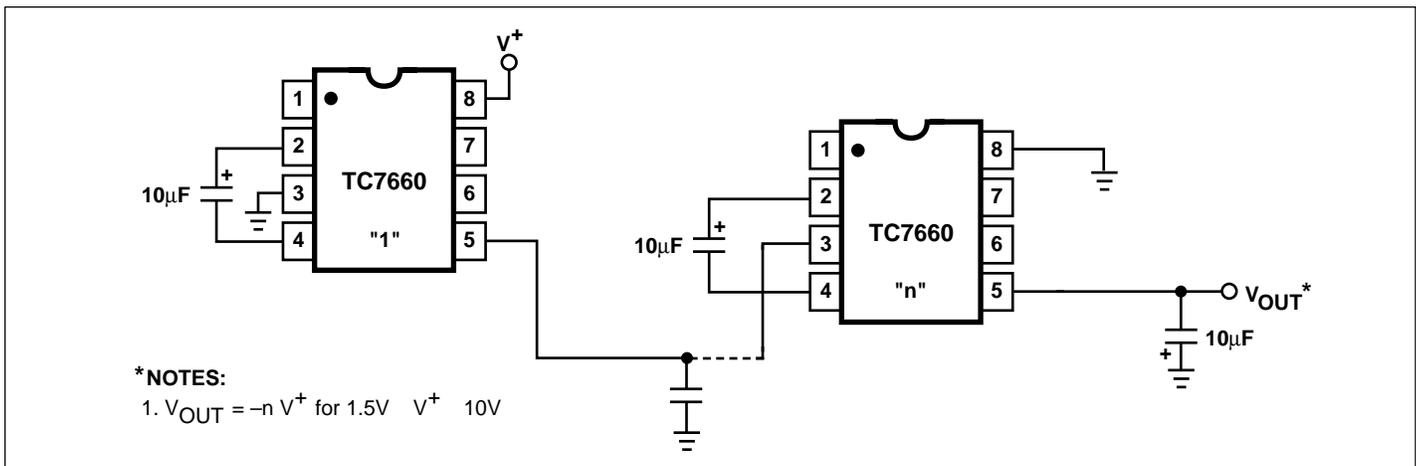
Figure 5. Increased Output Voltage by Cascading Devices
