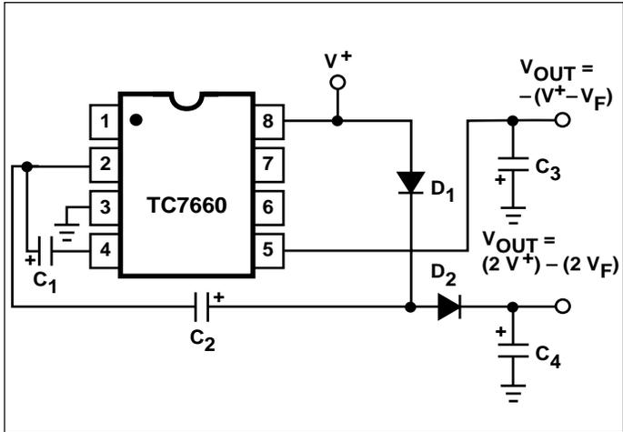
Figure 9. Combined Negative Converter and Positive Multiplier
