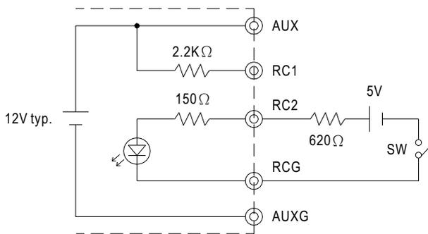
(B) Using internal 12V auxiliary output
