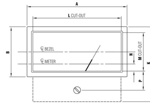
6.00mm/0.24" hole required when optional front zero is specified
