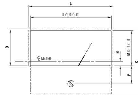
6.00mm/0.24" hole required when optional front zero is specified
