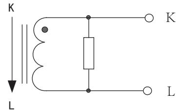
Voltage output type : Built-in with sampling resistance
