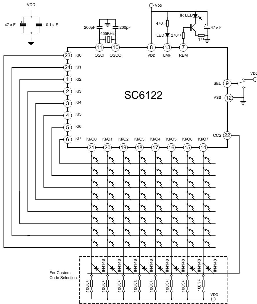
Note:1. Two capacitance connect with Vcc should as near as possible.
