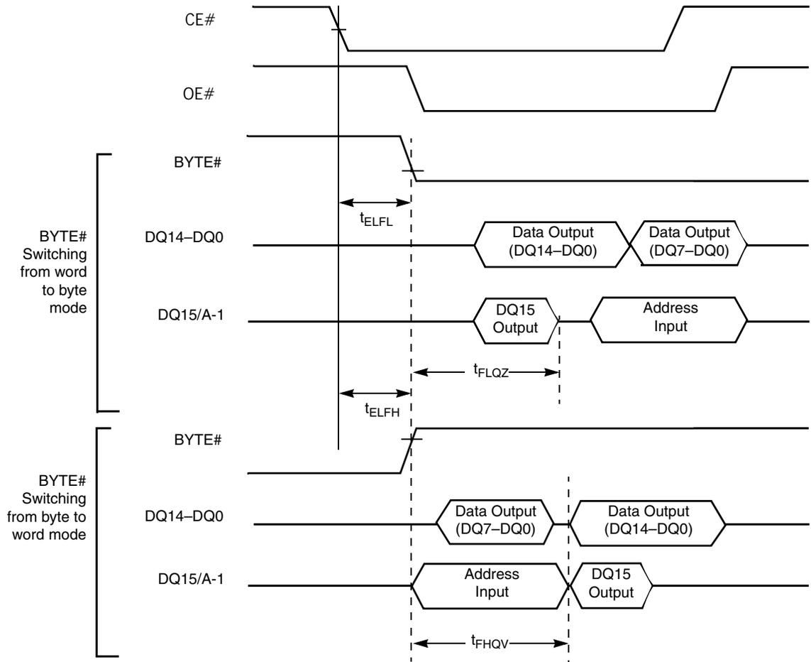
Figure 17.4 BYTE# Timings for Write Operations
