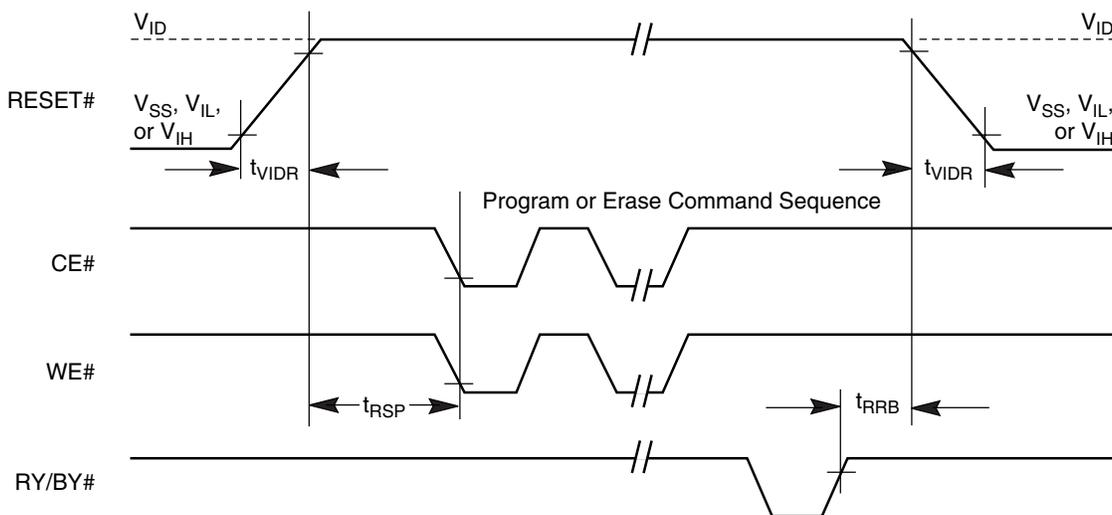
Figure 17.13 Sector/Sector Block Protect and Unprotect Timing Diagram
