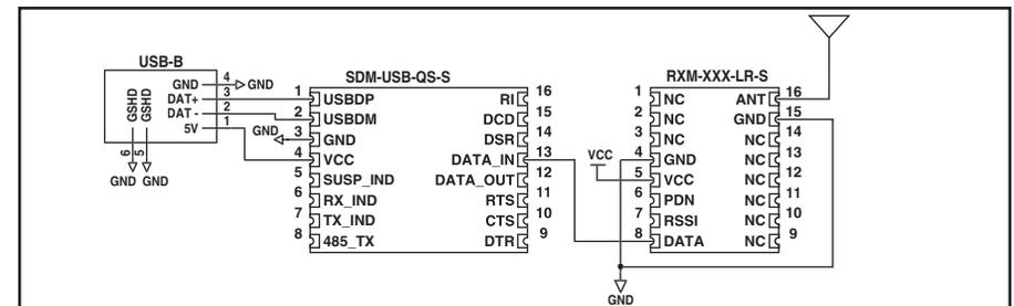
Figure 14: LR Receiver and Linx USB Module
