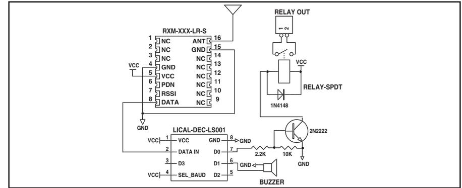
Figure 12: LR Receiver and LS Decoder
