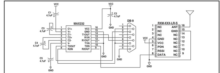
Figure 13: LR Receiver and MAX232 IC
