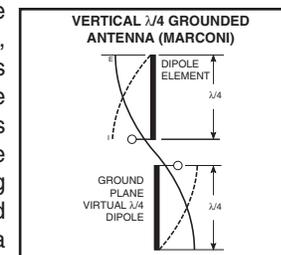
Figure 23: Dipole Antenna
