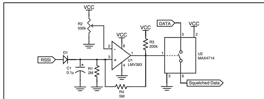
Figure 10: LR Receiver and LS Decoder
