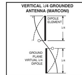
Figure 23: Dipole Antenna
