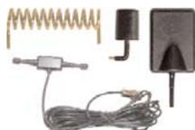
Linx offers a wide variety of specialized antenna styles. Many of these styles utilize helical elements to reduce the overall antenna size while maintaining reasonable performance. A helical antenna's bandwidth is often quite narrow and the antenna can detune in proximity to other objects, so care must be exercised in layout and placement.
