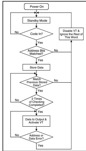
Figure 9: Decoder Flowchart
