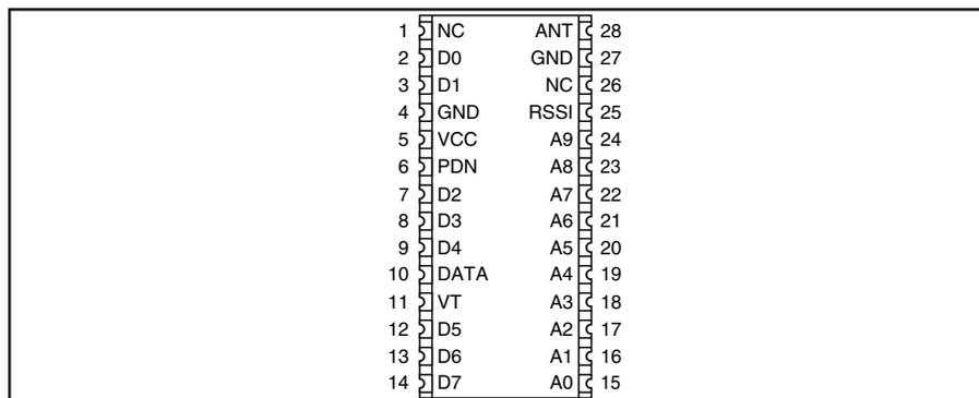
Figure 7: KH2 Series Receiver Pinout (Top View)
