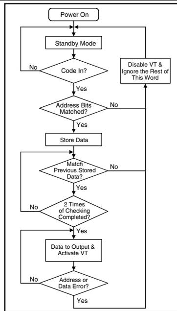
Figure 9: Decoder Flowchart
