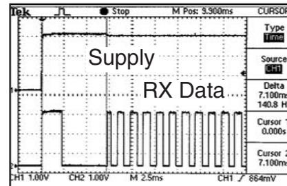
Figure 3: Turn-On Time from V<sub>CC</sub>
