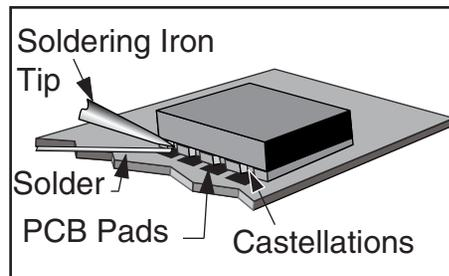
Figure 18: Soldering Technique
