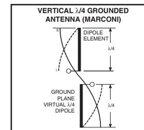
Figure 23: Dipole Antenna
