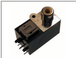
**OTJ-6/ORJ-6 Dual SPDIF RCA and Optical Transmitter and Receiver Jack. Right angle PCB mount with self tapping hole for panel mounting. Hinged shutter. Several different colored inserts available.**
