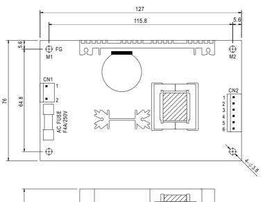
AC Input Connector (CN1): Molex 5277-02 or equivalent
