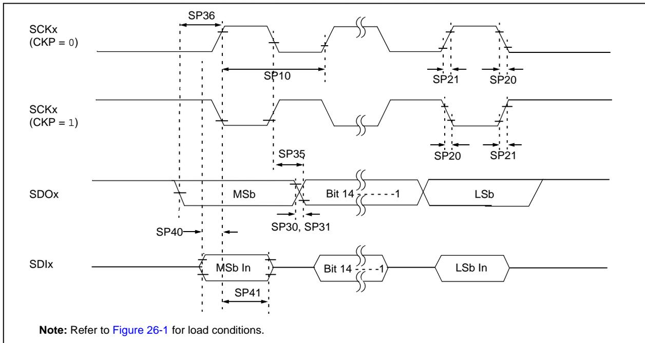
**TABLE 26-39: SPIx MASTER MODE (FULL-DUPLEX, CKE = 1, CKP = x, SMP = 1) TIMING REQUIREMENTS FOR PIC24FJ32MC101/102/104**
