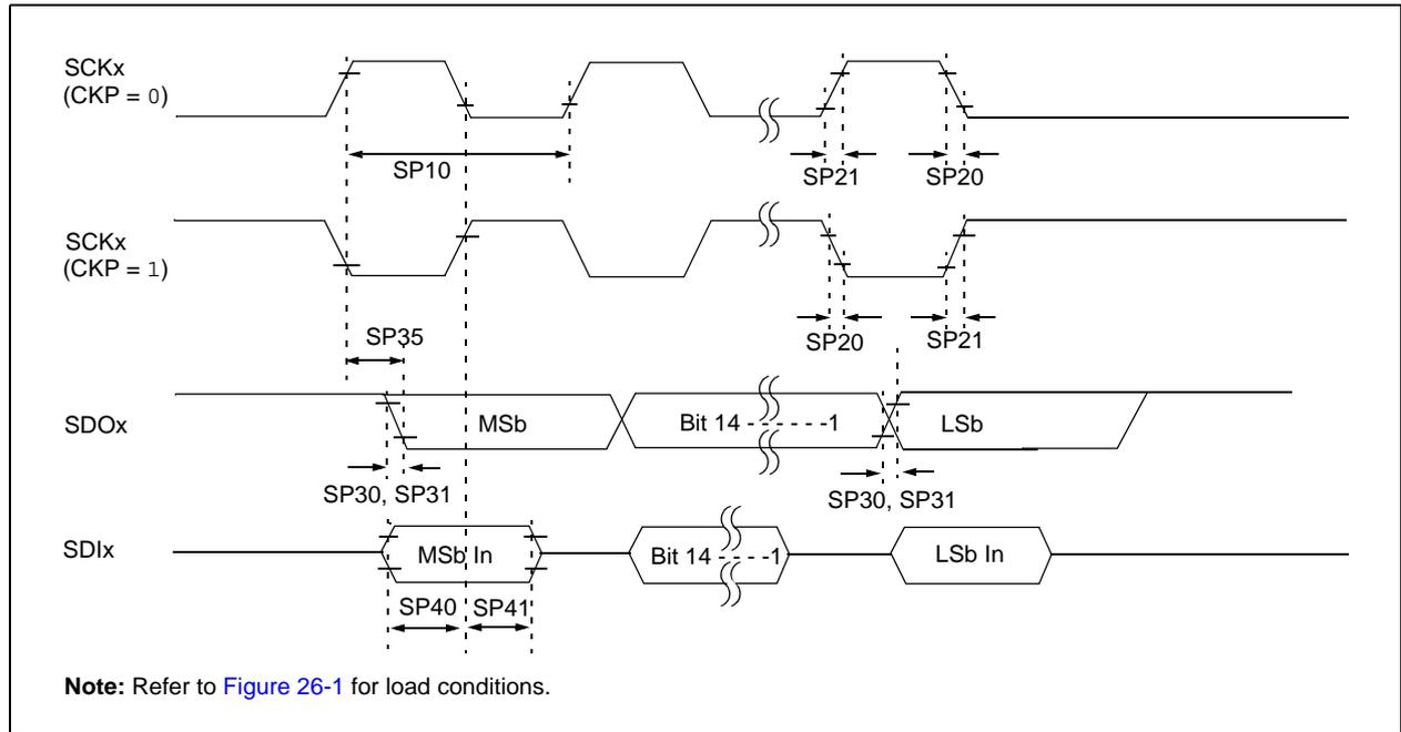
**TABLE 26-32: SPIx MASTER MODE (FULL-DUPLEX, CKE = 0, CKP = x, SMP = 1) TIMING REQUIREMENTS FOR PIC24FJ16MC101/102**
