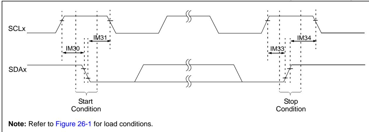
**FIGURE 26-28: I2Cx BUS DATA TIMING CHARACTERISTICS (MASTER MODE)**
