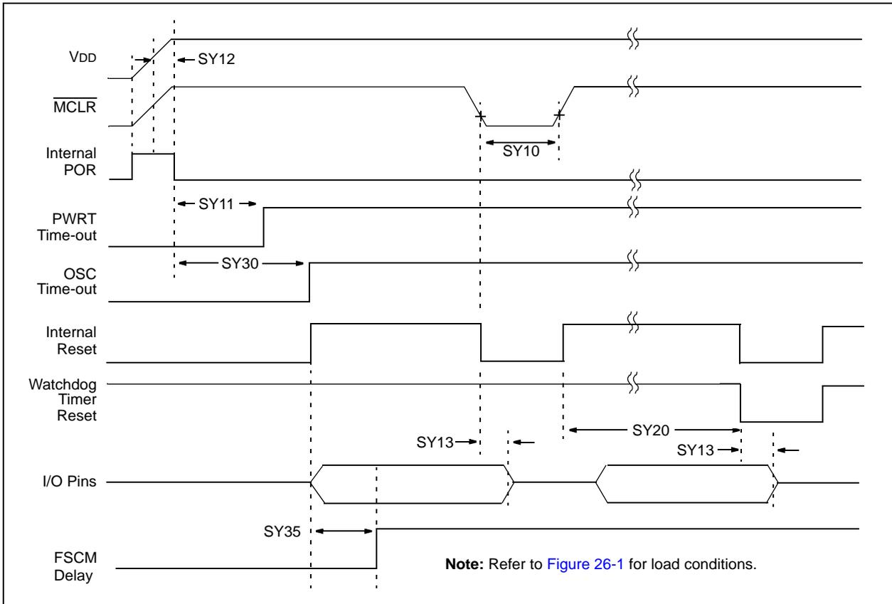
**TABLE 26-21: RESET, WATCHDOG TIMER, OSCILLATOR START-UP TIMER AND POWER-UP TIMER TIMING REQUIREMENTS**
