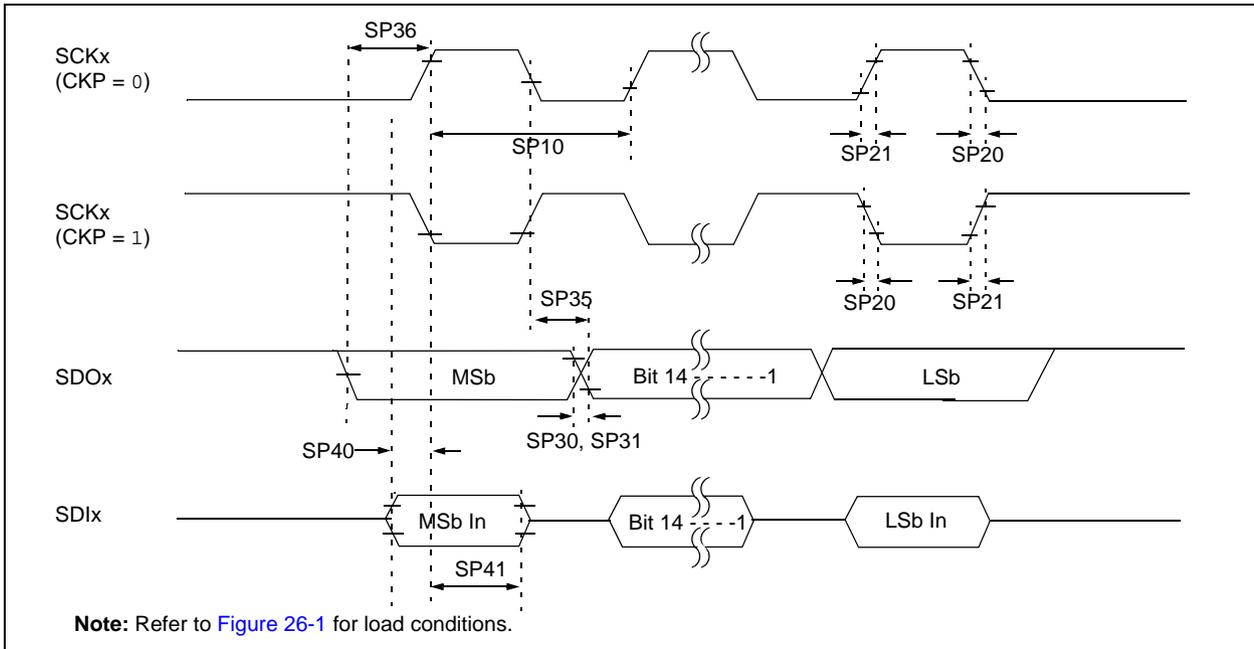
**TABLE 26-31: SPIx MASTER MODE (FULL-DUPLEX, CKE = 1, CKP = x, SMP = 1) TIMING REQUIREMENTS FOR PIC24FJ16MC101/102**
