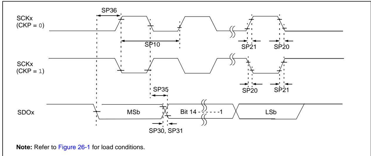
**TABLE 26-38: SPIx MASTER MODE (HALF-DUPLEX, TRANSMIT ONLY) TIMING REQUIREMENTS FOR PIC24FJ32MC101/102/104**
