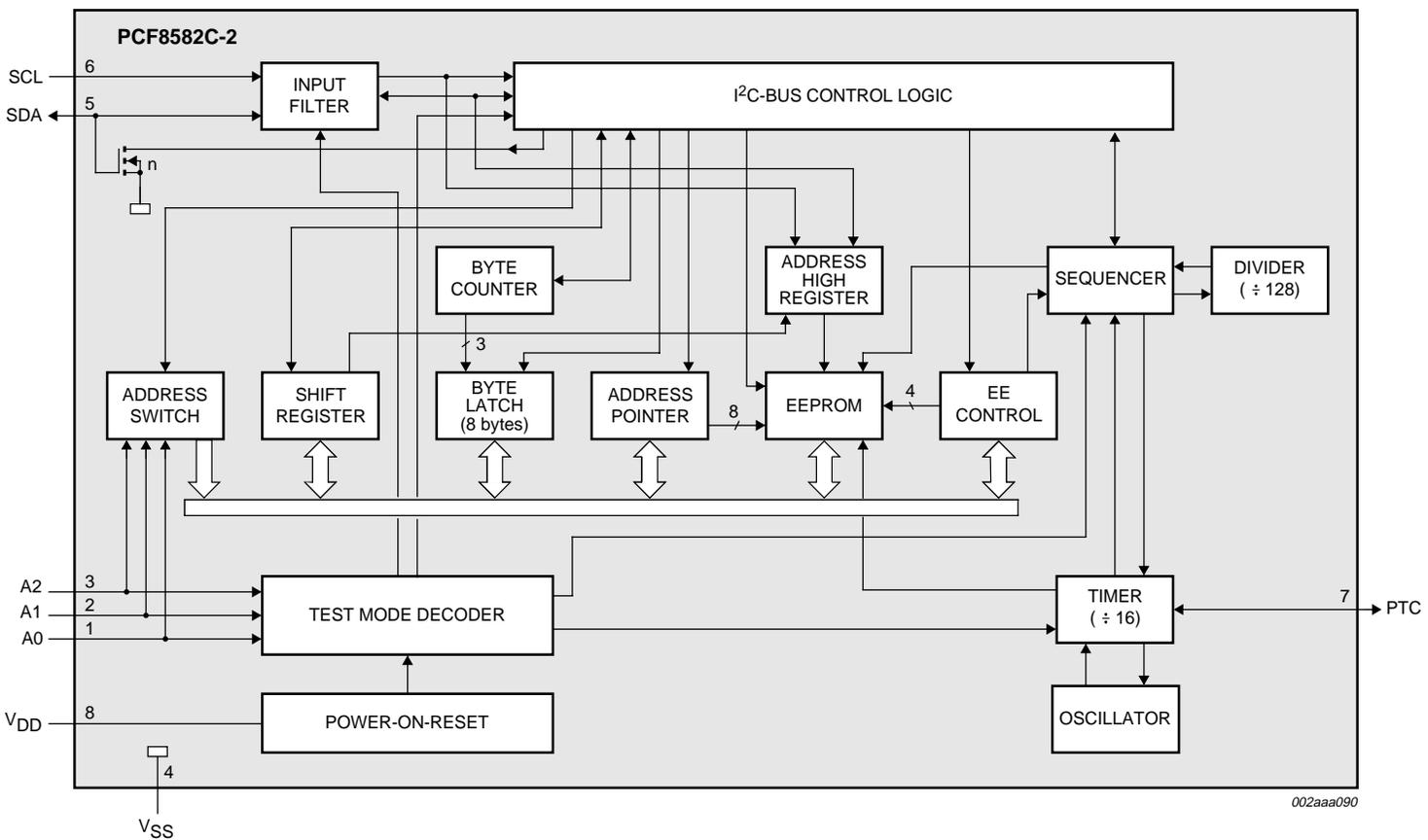
Fig 1. Block diagram.
