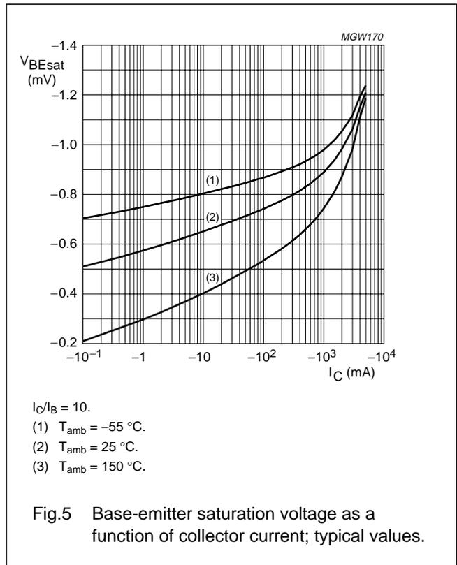
50 V low  $V_{CEsat}$  PNP transistor
