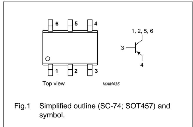
50 V low  $V_{CEsat}$  PNP transistor
