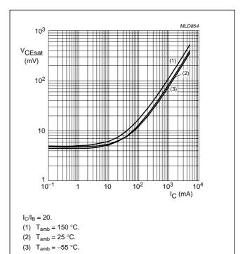
Collector-emitter saturation voltage as a
