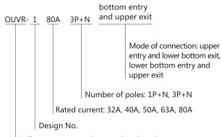
Self-recovery overvoltage and undervoltage protector
