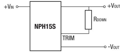
When the output voltage is trimmed up, output current must be derated so that the maximum output power is not exceeded.
