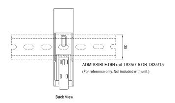
This series fits DIN rail TS35/7.5 or TS35/15. For installation details, please refer to the USER MANUAL on http://www.meanwell.com/search/NDR-75/NDR\_manual.pdf
