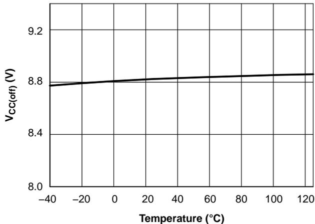
Figure 5. V<sub>CC(off)</sub> vs. Junction Temperature
