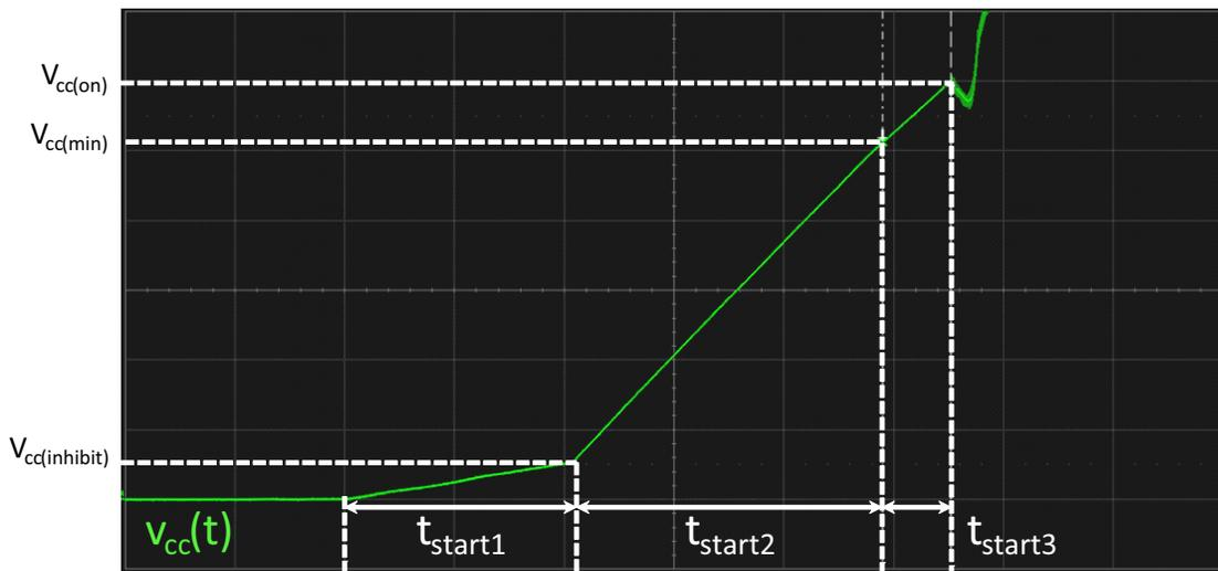
Figure 32. The V<sub>CC</sub> at Start-Up is Made of Two Segments Given the Short-Circuit Protection Implemented on the HV Source
