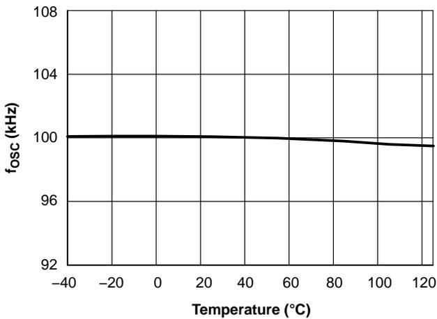
Figure 19.  $f_{OSC}$  (100-kHz Version) vs. Junction Temperature
