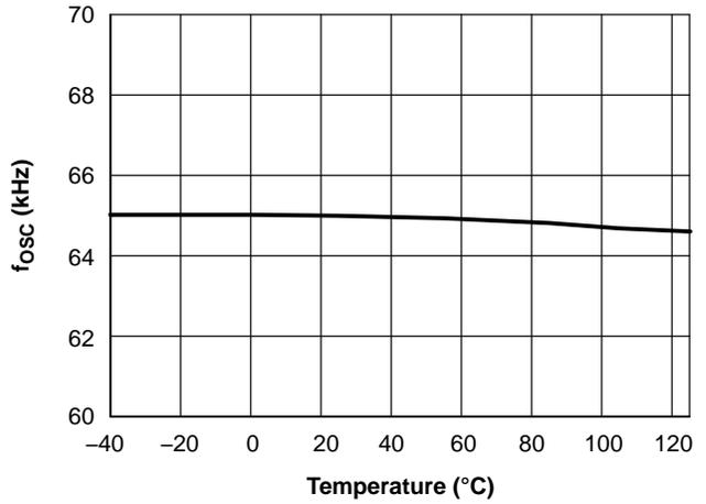
Figure 18.  $f_{OSC}$  (65-kHz Version) vs. Junction Temperature
