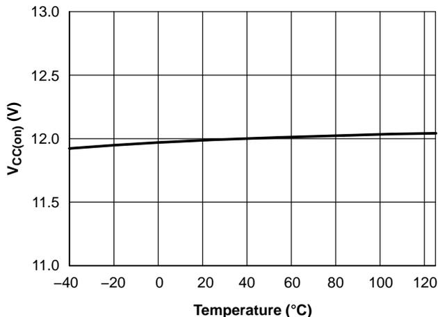
Figure 3. V<sub>CC(on)</sub> vs. Junction Temperature
