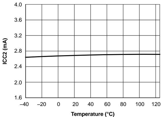
Figure 8. ICC2 (100-kHz Version) vs. Junction Temperature
