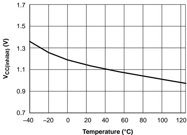
Figure 6. V<sub>CC(inhibit)</sub> vs. Junction Temperature
