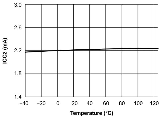
Figure 7. ICC2 (65-kHz Version) vs. Junction Temperature
