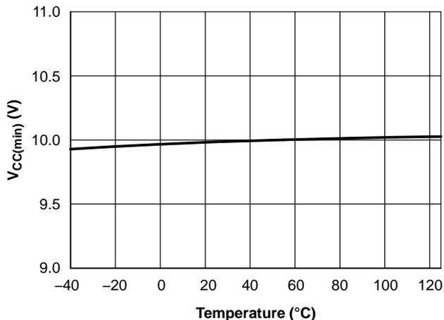
Figure 4. V<sub>CC(min)</sub> vs. Junction Temperature
