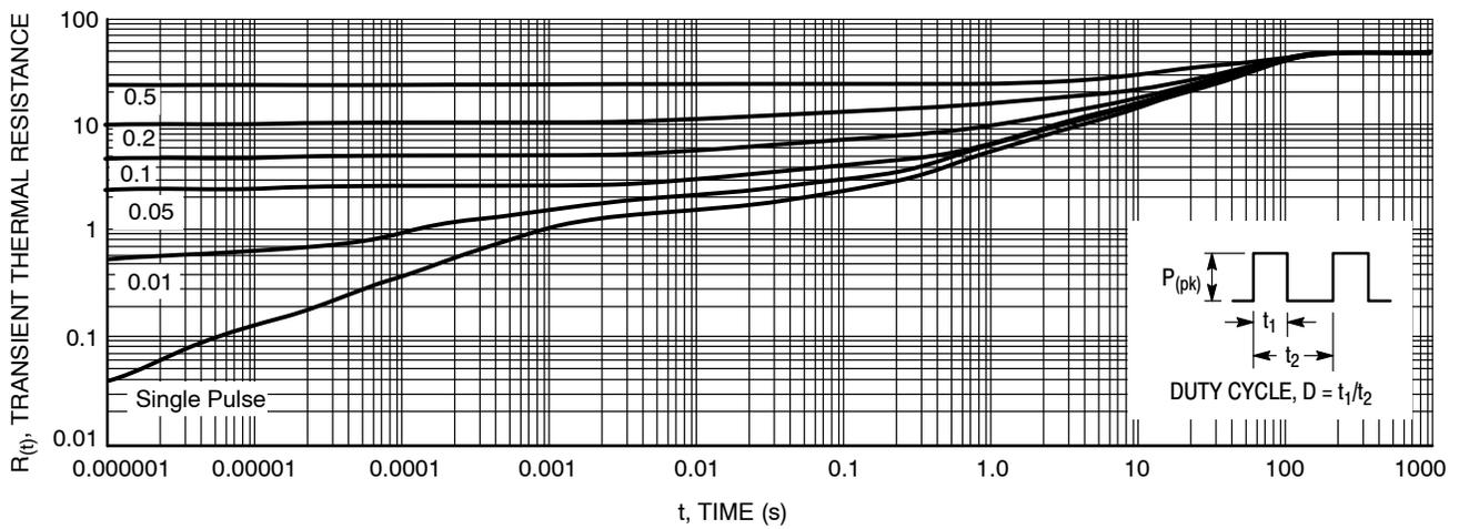
Figure 9. Thermal Response, Junction to Ambient
