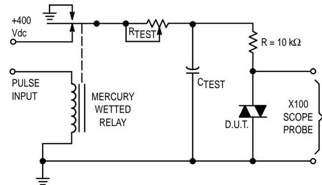
1. The mercury wetted relay provides a high speed repeated pulse to the D.U.T.
