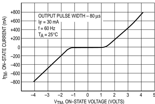
**Figure 1. On-State Characteristics**
