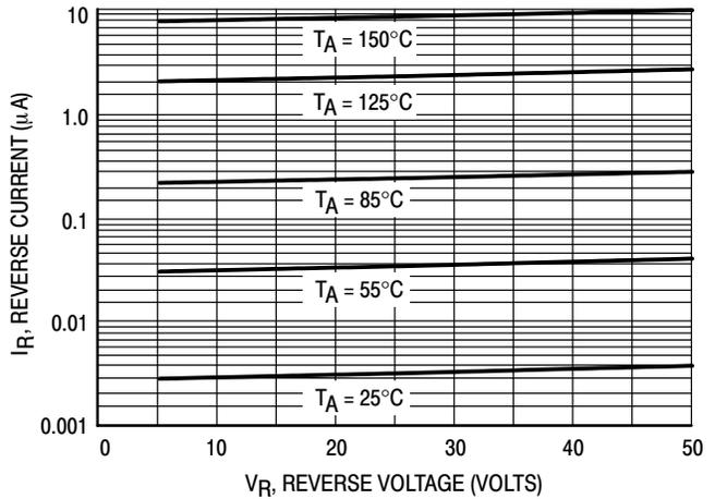
**Figure 3. Leakage Current**
