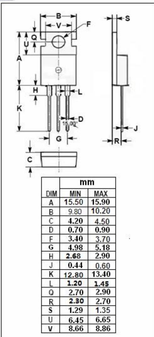
**isc Silicon PNP Power Transistor****MJE15031****ELECTRICAL CHARACTERISTICS****T<sub>c</sub>=25°C unless otherwise specified**
