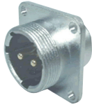
M595715 A / B / C / F CIRCULAR MALE M22 CONNECTOR (A)2P(B)3P-15A250V (C)4P(F)7P-10A250V
