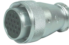
M595723 F / K / P / Q / T / Z CIRCULAR MALE M30 CONNECTOR (F) 7P-15A250V (K)12P-10A250V (P)16P(Q)17P(T)20P(Z)26P-5A250V
