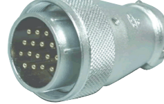
M595727 F / K / P / Q / T / Z CIRCULAR FEMALE M30 CONNECTOR (F) 7P-15A250V (K)12P-10A250V (P)16P(Q)17P(T)20P(Z)26P-5A250V
