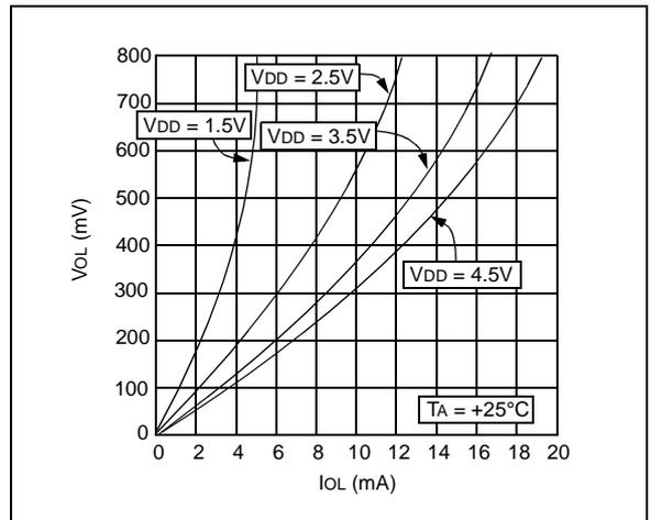
Figure 2-6: V<sub>OL</sub> vs. I<sub>OL</sub>
