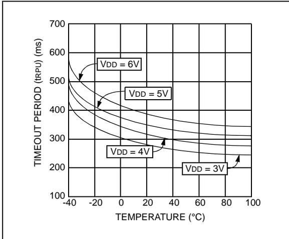
Figure 2-3: Typical t<sub>RP</sub> vs. Temperature
