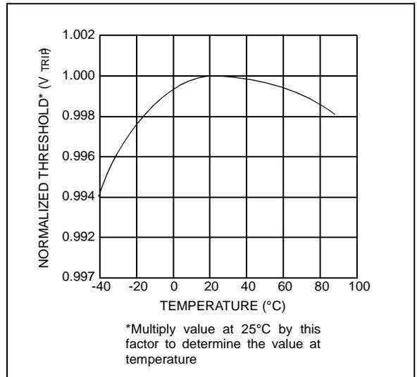
Figure 2-5: Normalized V<sub>TRIP</sub> vs. Temperature
