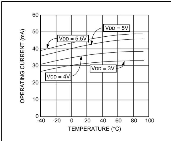
Figure 2-4: I<sub>DD</sub> vs. Temperature
