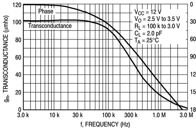
Figure 6. Error Amp Transconductance and Phase versus Frequency
