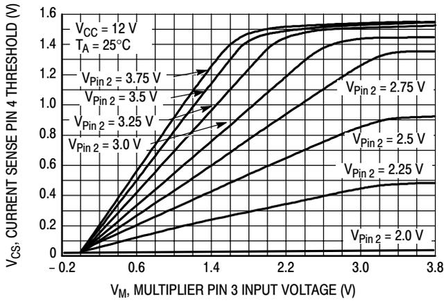
Figure 2. Current Sense Input Threshold versus Multiplier Input
