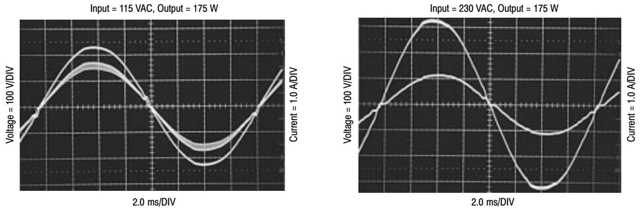
**Figure 23. Power Factor Corrected Input Waveforms (Figure 20 Circuit)**
