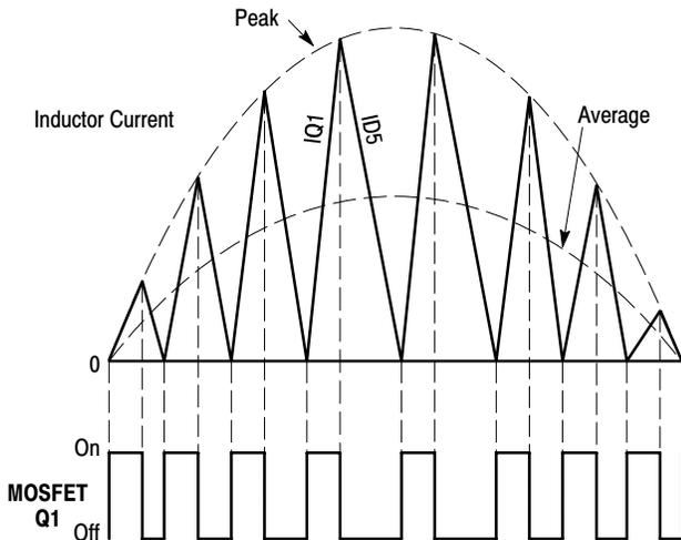
**Figure 19. Inductor Current and MOSFET Gate Voltage Waveforms**
