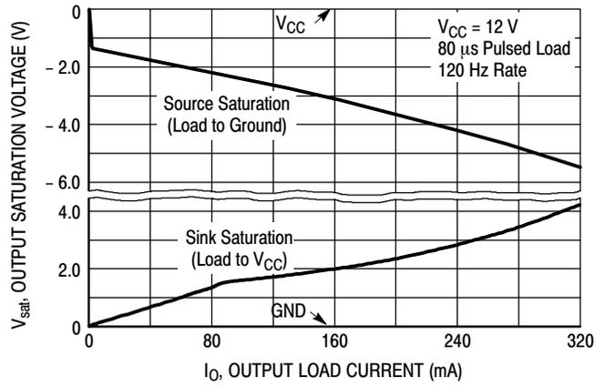
Figure 11. Output Saturation Voltage versus Load Current
