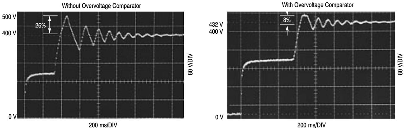
**Figure 24. Output Voltage Startup Overshoot (Figure 20 Circuit)**
