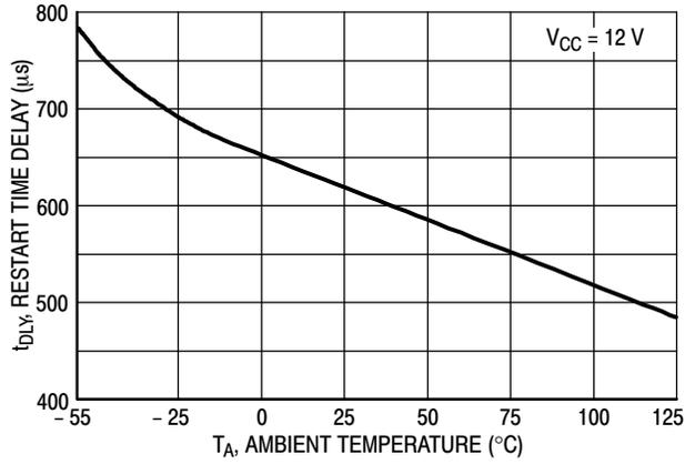
Figure 9. Restart Timer Delay versus Temperature
