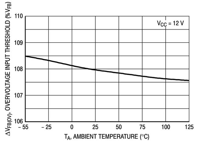
Figure 5. Overvoltage Comparator Input Threshold versus Temperature
