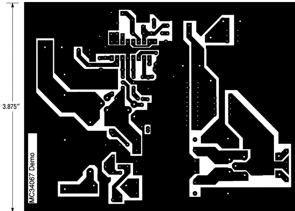
Figure 23. Printed Circuit Board and Component Layout
