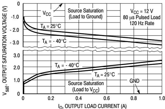
Figure 9. Drive Output Saturation Voltage versus Load Current
