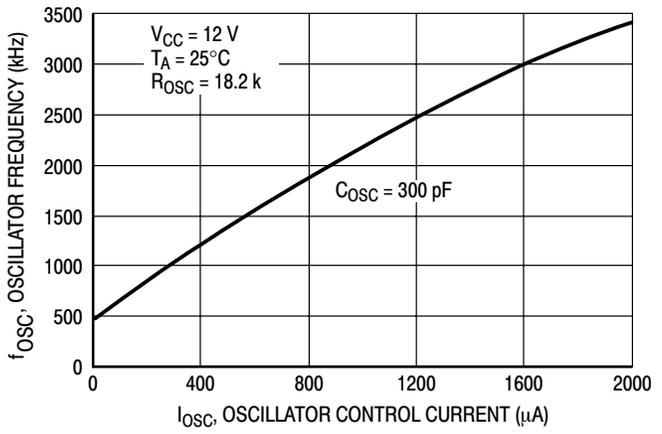
Figure 3. Oscillator Frequency versus Oscillator Control Current
