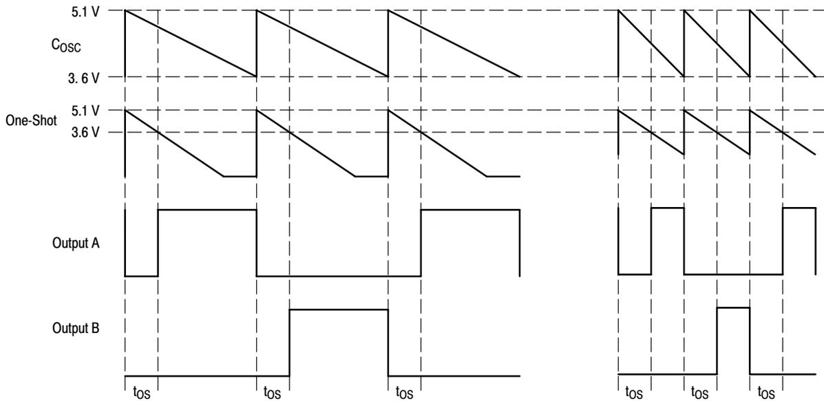
High State Error Amp output, minimum  $I_{OSC}$  current occurring at minimum input voltage, maximum load.
