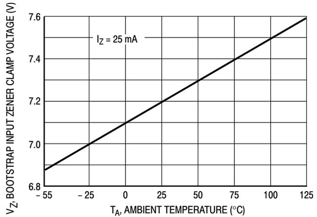
Figure 7. Bootstrap Input Zener Clamp Voltage versus Temperature
