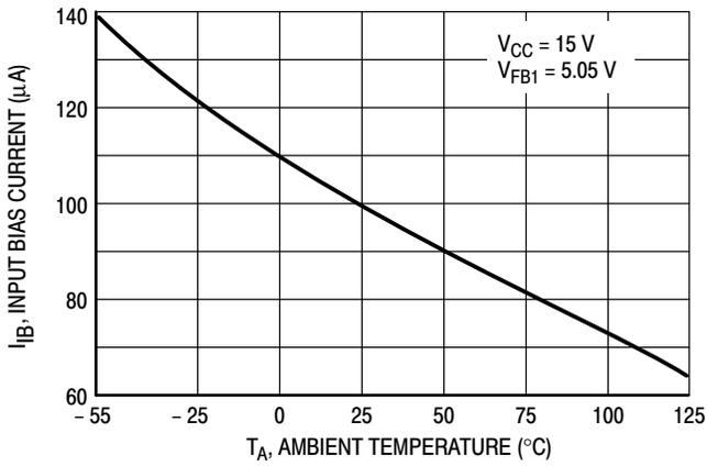
Figure 4. Feedback Comparator 1 Input Bias Current versus Temperature
