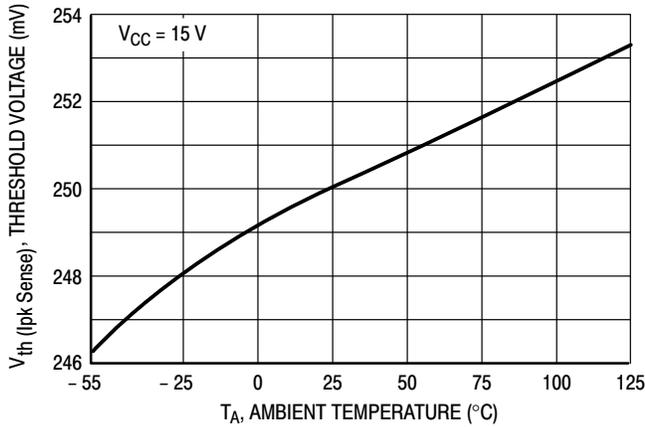
**Figure 12. Current Limit Comparator Threshold Voltage versus Temperature**
