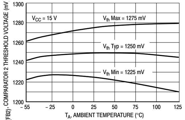
Figure 5. Feedback Comparator 2 Threshold Voltage versus Temperature
