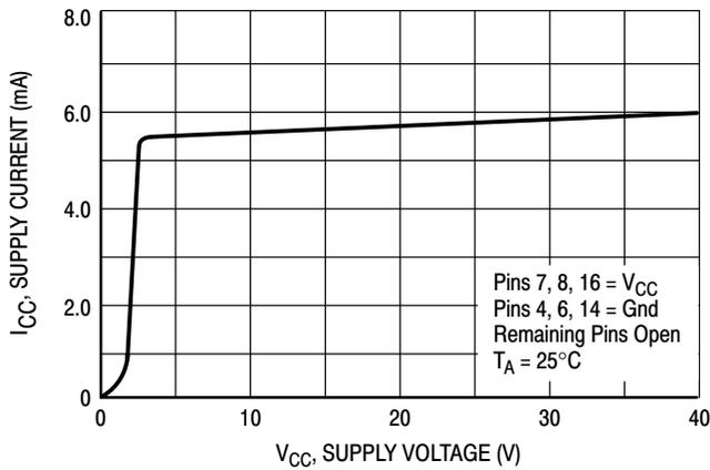
**Figure 14. Standby Supply Current versus Supply Voltage**
