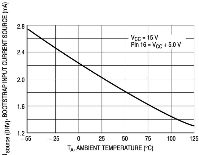
Figure 6. Bootstrap Input Current Source versus Temperature
