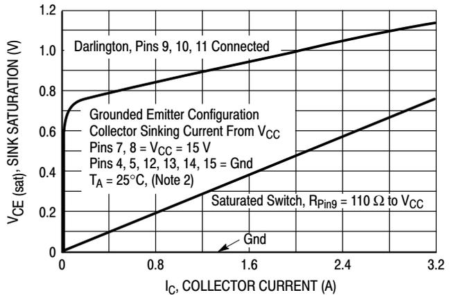
Figure 9. Output Switch Sink Saturation versus Collector Current
