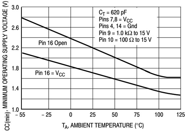
**Figure 16. Minimum Operating Supply Voltage versus Temperature**
