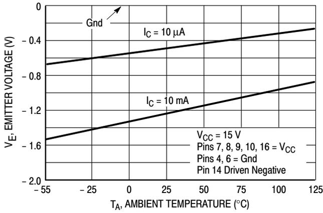
**Figure 10. Output Switch Negative Emitter Voltage versus Temperature**
