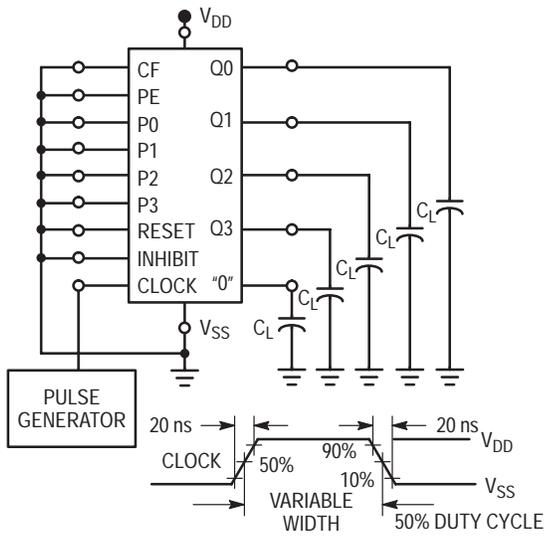
Figure 3. Power Dissipation
