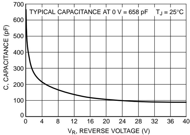
Figure 7. Typical Capacitance
