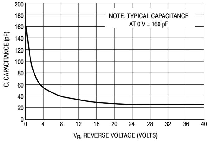
Figure 3. Typical Capacitance
