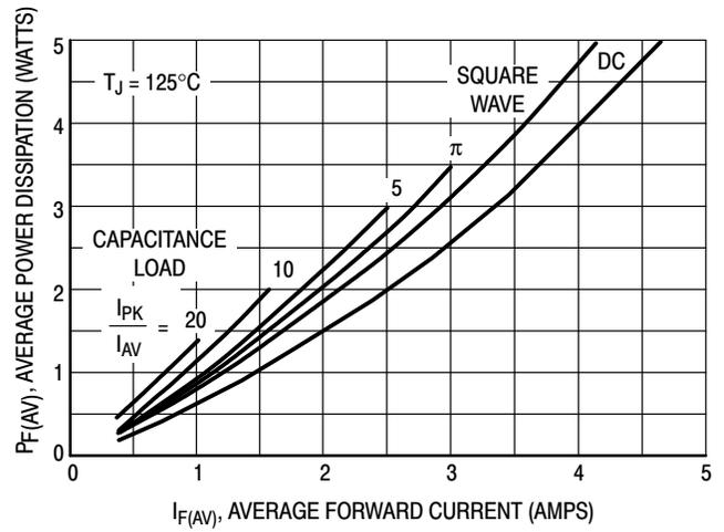
Figure 5. Power Dissipation
