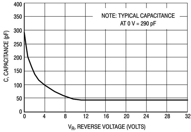
Figure 5. Typical Capacitance
