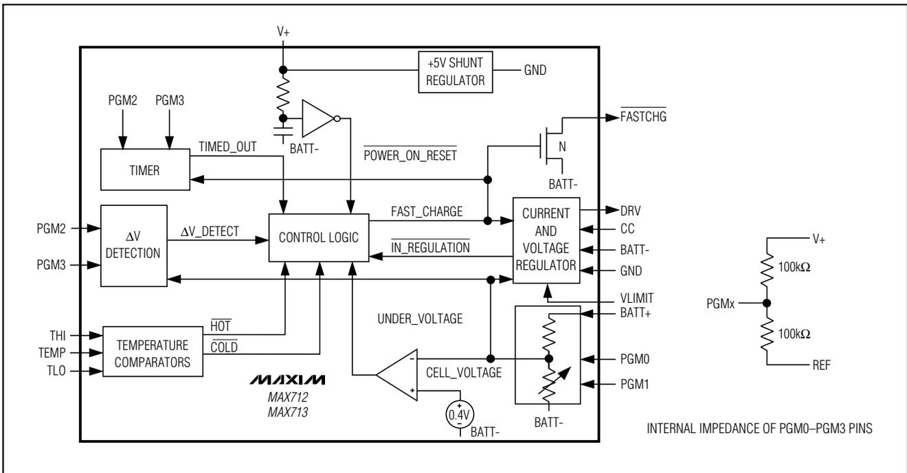
Figure 1. Block Diagram
