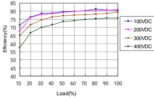
LS03 DC input rated load efficiency cure
