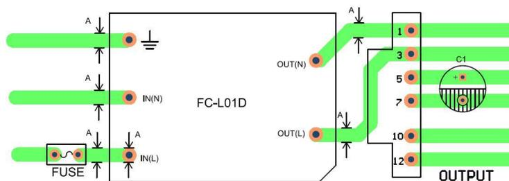
Figure 4: EMC application circuit PCB layout
