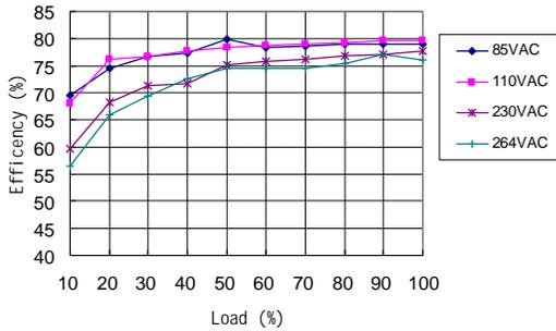
LS03 AC input rated load efficiency cure
