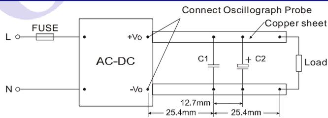
Note: C1: 1μF (Ceramic capacitor) C2: 10μF (Electrolytic capacitor)
