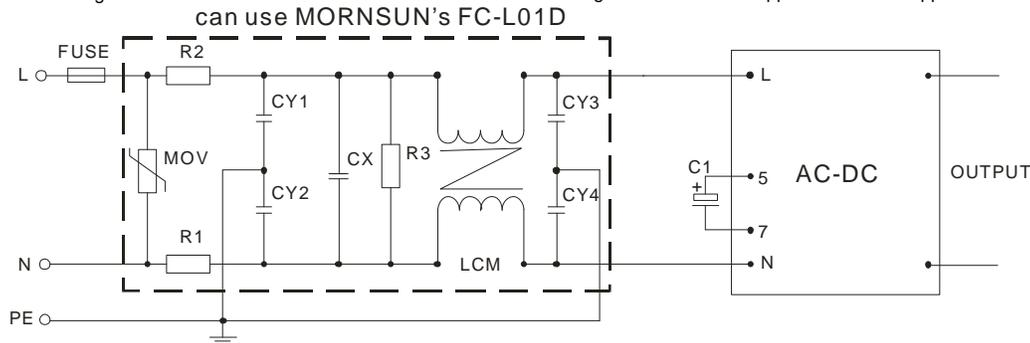
Figure 3: LS03-R2 series Recommended circuit for application require higher EMC standard (external circuit output same as above)
