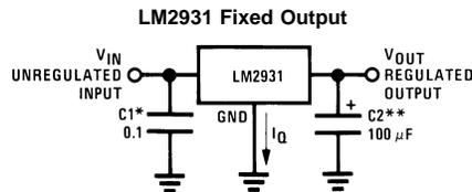
\*Required if regulator is located far from power supply filter.
