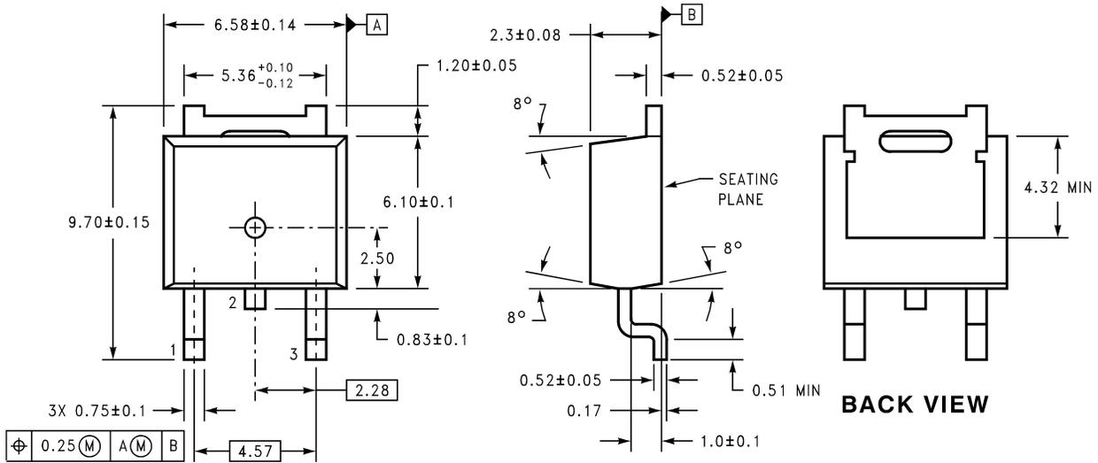
**DIMENSIONS ARE IN MILLIMETERS**
