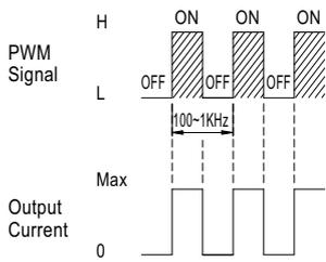
⊙ During PWM dimming operation, the output current will change to PWM style.
