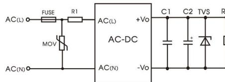
Fig. 2: EMC application circuit with higher requirements
