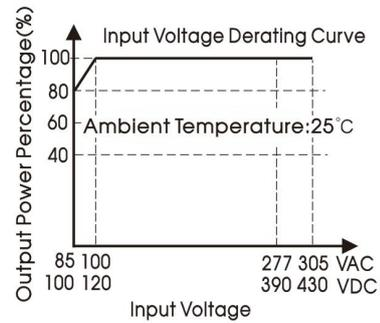
Note: ① With an AC input between 85-100V a DC input between 100-120VDC, the output power must be derated as per temperature derating curves;
