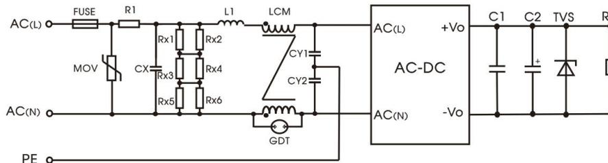
Fig. 3: Recommended circuit for class I equipment
