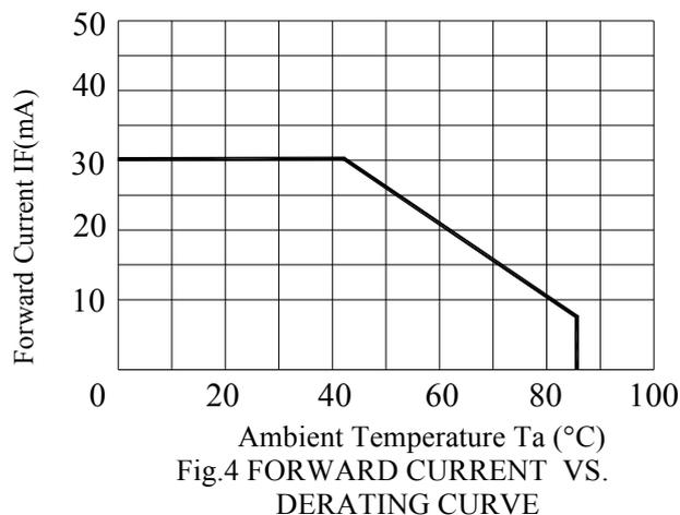
Fig.4 FORWARD CURRENT VS. DERATING CURVE
