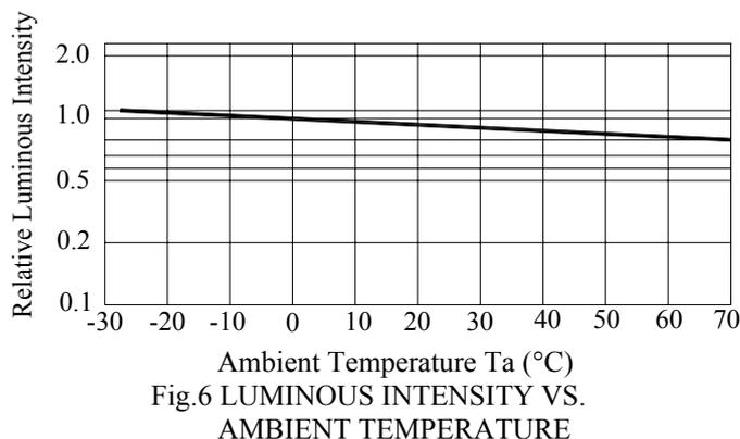
Fig.6 LUMINOUS INTENSITY VS. AMBIENT TEMPERATURE
