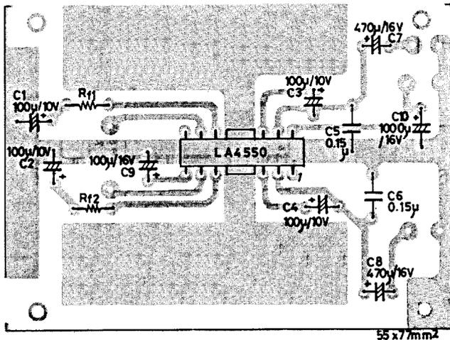
Sample Printed Circuit Pattern (Cu-foiled area) for Stereo Use
