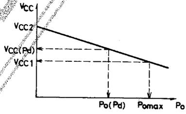
$$Pd \text{ max} = \frac{V_{CC}(Pd)^2}{\pi^2 R_L} + I_{CC0} \cdot V_{CC} (Pd) \quad (\text{For stereo use}) \dots (2)$$
