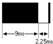
Note: after the pulse waveform is integrated into the receiving head, it is decoding, signal amplifying and shaping in the integrated receiver head, therefore, should pay attention to: in the absence of infrared signal, its output is high level and voce vice. The output signal level is opposite to emission port. The receiving port pulse we can see through the oscilloscope, so understand the program with waveform.
