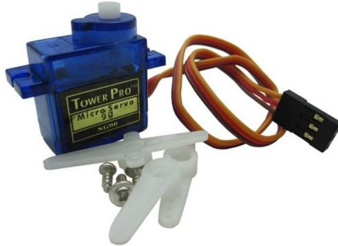
The servo has many specifications, but all of the actuator is connected respectively with three lines, brown, red, orange three colors to distinguish, as the servo with different brand, color will vary, brown for the ground line, red for the positive power supply line, orange for the signal line.
