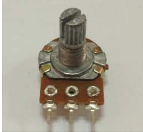
In this experiment, we will turn potentiometer resistance into analog values read out, and then display on the screen. This is the example of the application that we are also required to master when we need to complete our own experiment functions. We must first connect
