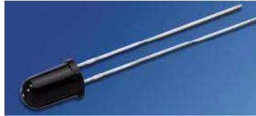
The flame sensor (i.e. the infrared receiver) is used to search for the heat source for robot. The sensor is especially sensitive to the flame.
