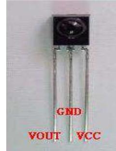
When Connect the VOUT to analog port, GND connects to the GND on experimental panel, VCC connects to the +5v on the experimental panel.
