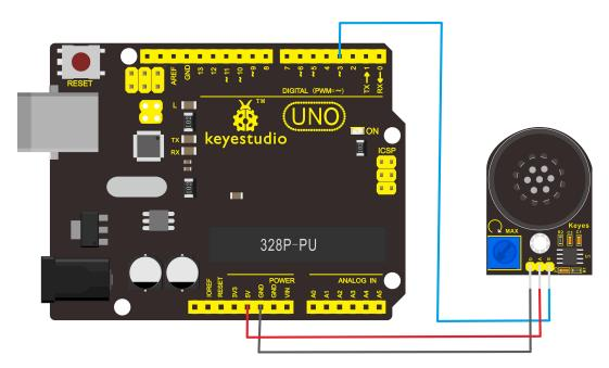
Connect the power amplifier module to control board using three jumper wires.
